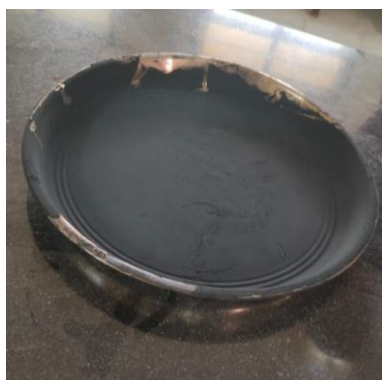
Fig 13: Black soot deposited on steel plate
